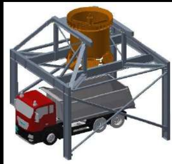
WLL: 27 Tonne (12.5 cu.m) Direct to Truck
