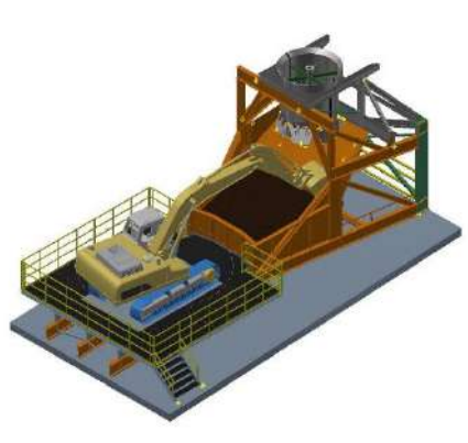
Capacity :60t (25 cu.m) CAT336, 12.5cu Kibble
