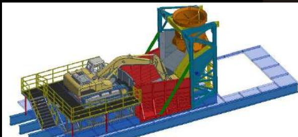
Capacity :160t (65 cu.m) CAT336, 17.5cu Kibble operator
