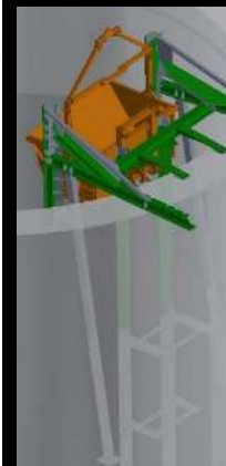
WLL: 19 Tonne (12.5 cu.m) Rail-guided, Self-tipping by Crane
