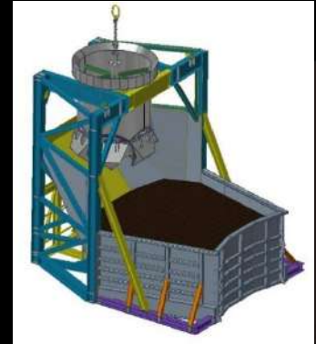
Capacity :60t (25 cu.m) Freestand, 17.5cu Kibble
